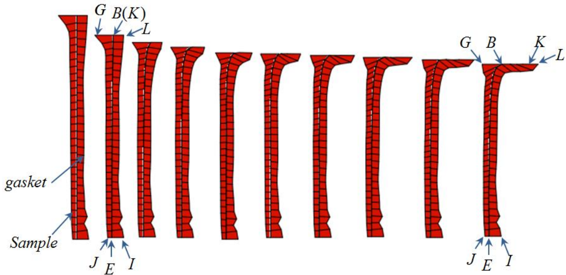
FIG. 8. Extrusion-based pseudoslip as the mechanism of sliding at the contact line (line GBL ) between sample (left to the curve BE ), gasket (right to the curve BE ), and anvil (line GBL ) during compression. Initially, points B of the sample and K of the gasket coincide. The evolution of geometry of two layers of finite elements along the contact surface ( BE ) in Fig. 1(d) during compression. Point L of gasket does not slide along the anvil because the sliding condition for it is not met, while sliding condition for points of the sample is satisfied. Sample sliding with respect to the anvil is possible because of the sliding of the gasket material along the sample and its extrusion, which produces a new gasket-anvil contact surface ( BK ).
